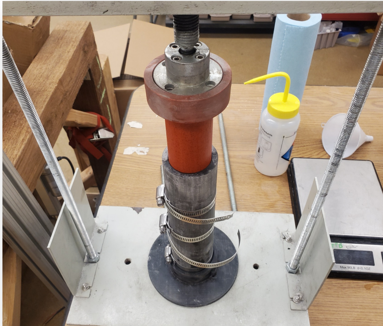
Core Press/Mold Used to Manufacture Tested Cores
