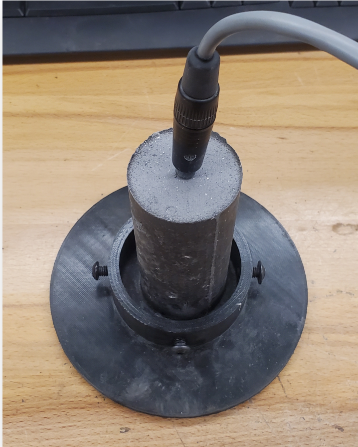
Thermal Conductivity Test Using a MP-2 Thermal Conductivity Probe
