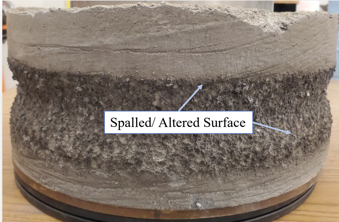
Nectar A Simulant “Cake” Post Test 353.4 W/cm 2 Avg. Irr. at FWHM size
