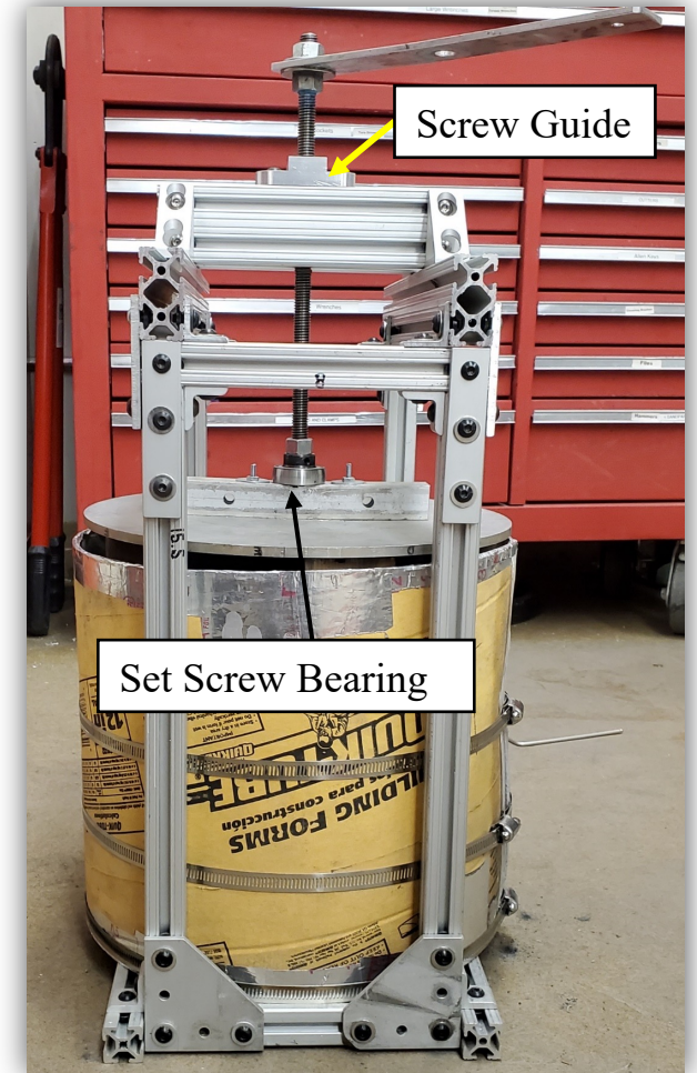
Load Press for Nectar Cake Simulant Production
